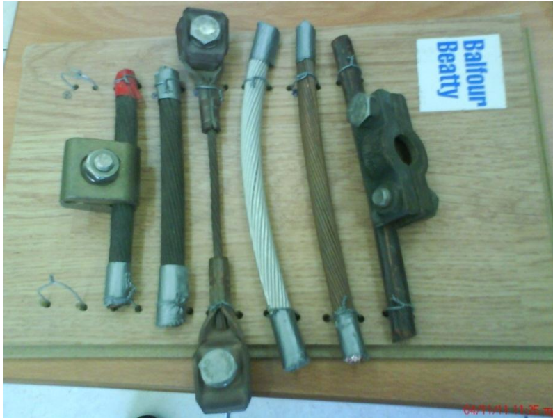
Image 1 Types of copper and aluminium cables that are stolen from Railway
